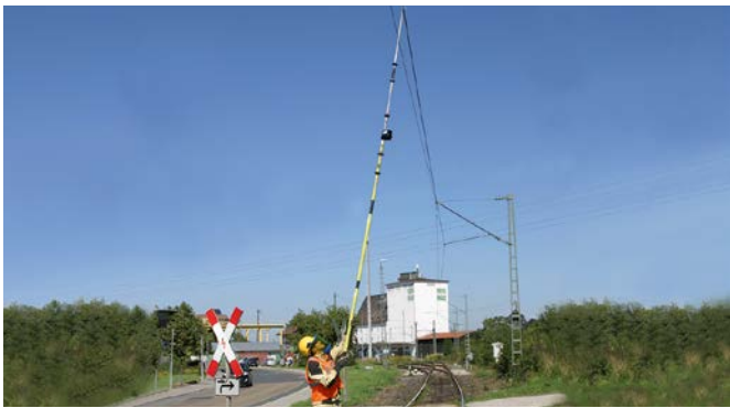
PHE voltage detector with visual indicator used on an overhead contact line of German Railways (DB).
