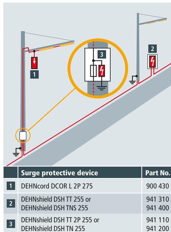
Figure 3 Combined arrester installed in the terminal compartment/distributor of the metal mast in conjunction with a surge arrester for protecting the LED mast light from nearby atmospheric events and conducted surges caused by switching operations
