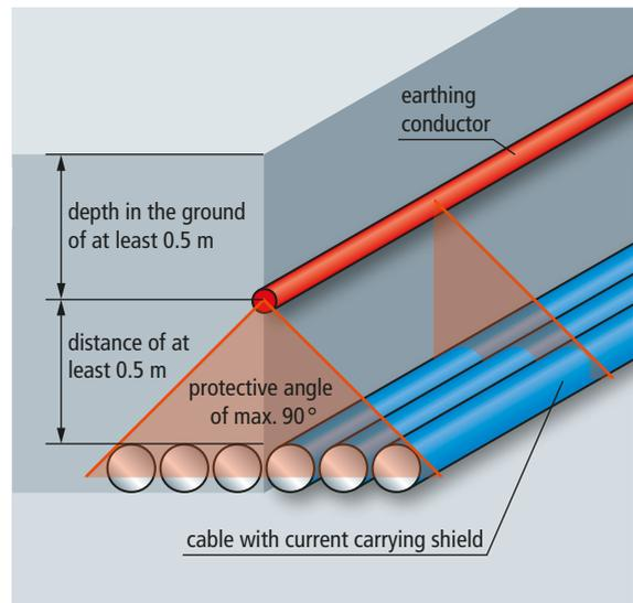
Figure 5 Protected zone of a cable route
