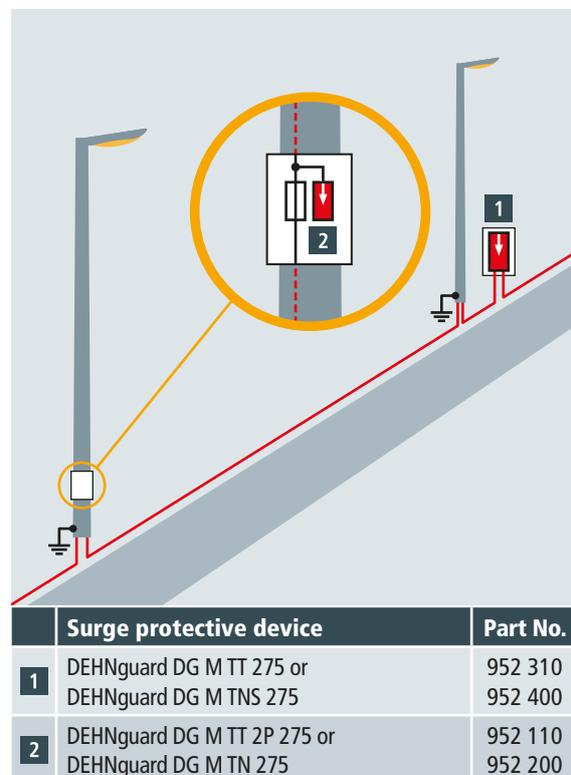
Figure 1 Surge arrester installed in the terminal compartment / distributor of the metal mast for protecting the metal LED mast light from conducted surges caused by distant atmospheric events and switching operations
