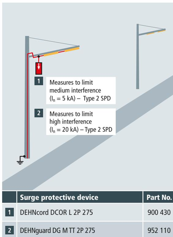
Figure 2 Surge arrester installed next to the LED mast light with the feeder cable of the mast light being installed in open space for protecting the LED mast light from field-based injection or as sole protection from conducted surges caused by distant atmospheric events and switching operations
