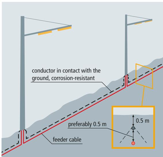
Figure 4 Earthing conductor for protecting the cable route and earthing the mast
